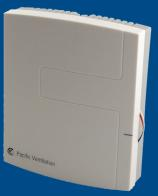
The controller compares room temperature with an adjustable set point and regulates a 0..10 V output signal applied to a ventilator with a PI algorithm in direct or reverse action based on jumper JP1 setting:
